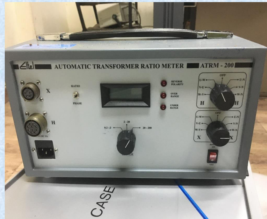
Transformer Turns Ratio Meter, Ratio range 0.2 to 200 turns, Accuracy 0.1 % FSD
